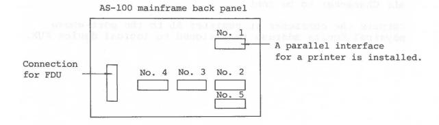
The user may install additional printer interfaces in ports #2 to #5. These ports are assigned the following physical device names:
